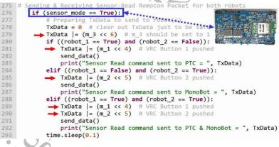
Fig. 3.134 Part 1 of the Sensor Read Procedure in "PTC\_MB\_ZGB\_Central.py".
