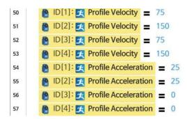
Fig. 2.13 Values used for Profile Velocities and Accelerations in "SBwA PositionControl 3 mm.tsk3".
