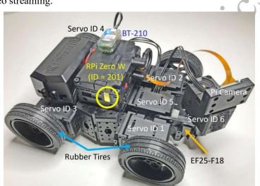
Fig. 3.1 Pan-Tilt Commando (PTC) robot with RPi0W and Pi Camera.
