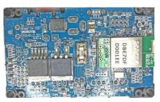
Fig. 1.1 Bottom view of CM-550 showing the embedded BT-410 module on the right.
