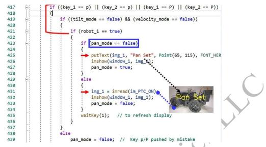
Fig. 3.189 Image and Text procedures for PTC's Pan mode in "PTC\_MB\_ZGB\_Central\_Relay.cpp".
