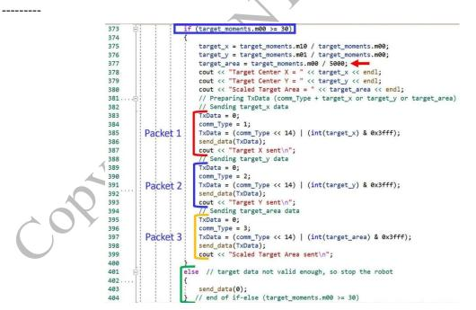
Fig. 3.174 Procedures used to send Target Pixel Area and Screen Coordinates X/Y to PTC in "PTC\_RC\_Color\_Tracker\_XY.cpp".
