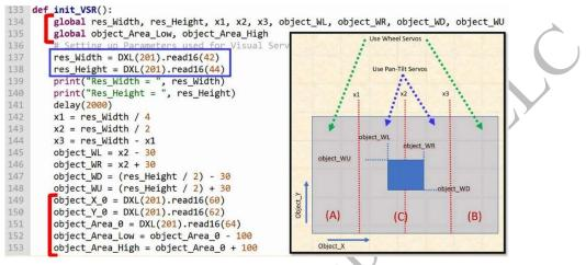
Fig. 3.78 Parameters used in the VSR Algorithm of "PTC\_RC\_VSR\_SD\_RPi\_CD.py".
