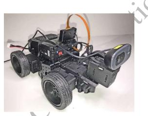
Fig. 3.104 PTC Robot with Logitech C270 Web Cam in "PTC\_RC\_Color\_Tracker\_XY.py".
