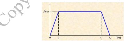
Fig. 2.20 Velocity Trajectory definition for a Time-Based Position Control option
