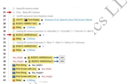
Fig. 3.23 Part 2 of Main Function in "PTC\_RC\_VSR\_SD\_RPi\_CD.tsk3".
