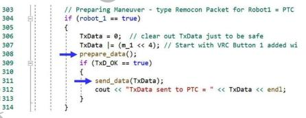
Fig. 3.184 Inserting Robot 1 ID into Remocon Message in "PTC\_MB\_ZGB\_Central.cpp".
